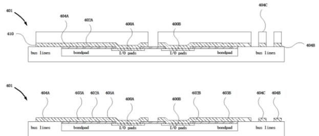
Fig. 4 (D-E) Cross-section view of Al layer lay up
