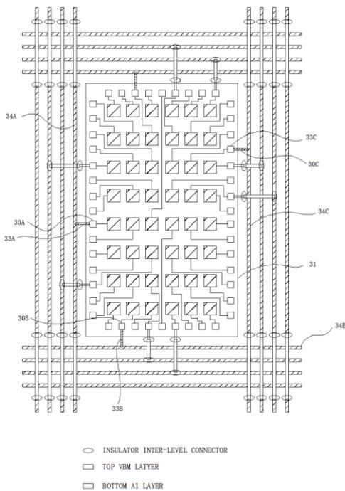
Fig. 3 Layout of signal buss to the assigned pin in the PGA configuration
