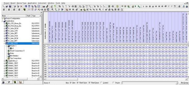
Fig. 9 Interconnection test checking the MCU related data, address and control buss
