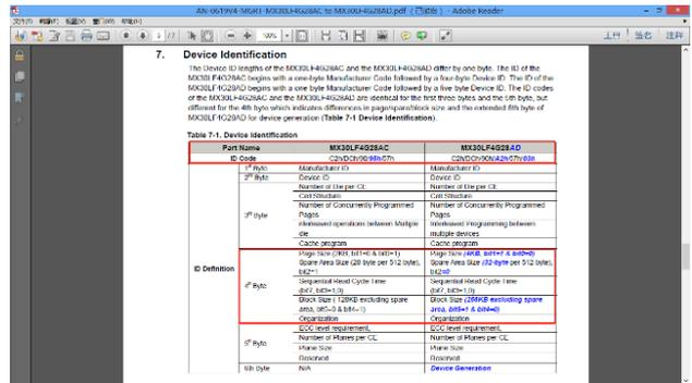
Picture 9. Attention made to data bus of a NAND flash memory for ID test
