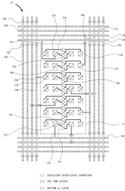
Fig. 2 Layout of 4x TAP signals across the die, embedded in the dicing streets and alleys
