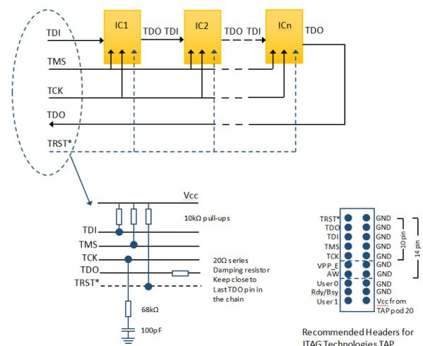
Picture 1. Boundary Scan based TAP port (Courtesy of JTAG Technologies)
