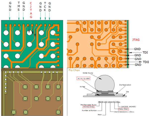
Picture 6. Illustrated examples of bumping process in rerouting
