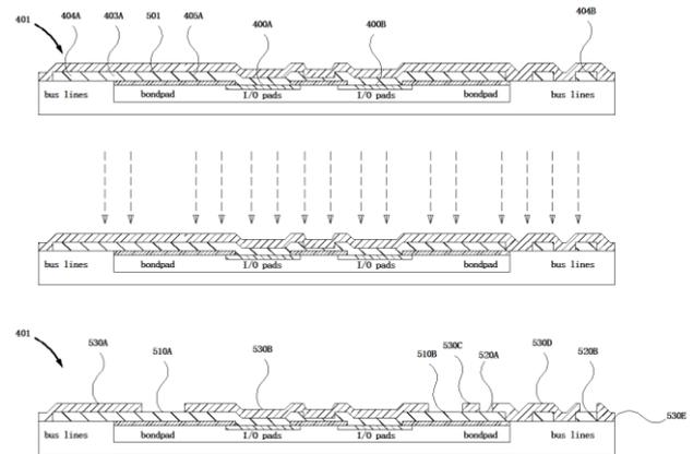
Fig.5 (5A-5C) side cross-sectional views of passivation
