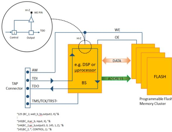
Picture 2. Boundary scan testing daisy chained dies (Courtesy of JTAG Technologies)
