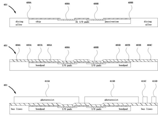
Fig. 4 (A-B-C) Cross-section view of dielectric layer lay-up
