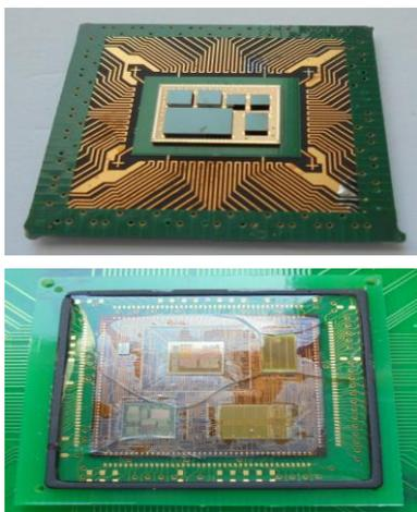
Picture 3. Prototyping Flip Chip based Multi-Chip-Module (Courtesy of JTAG Technologies)
