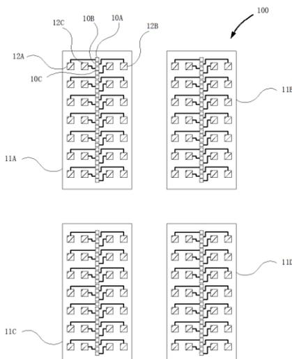
Fig. 1 Reconfigured Line of Centre (LOC) to Pin Grid Array (PGA)
