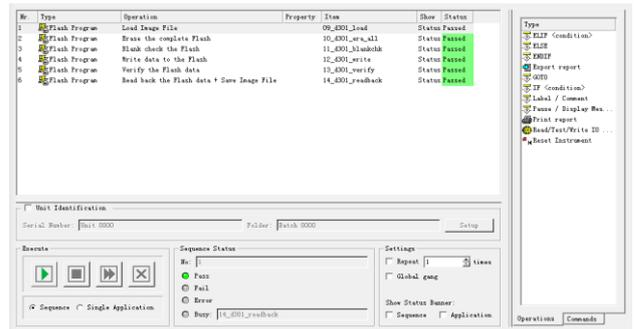
Fig. 11 step 2: Flash memory under erasing, blank checking, writing and verification
